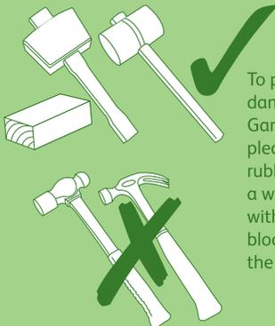
To prevent damage to the Garden Ring please use only a rubber mallet or a wooden mallet with a timber block to knock in the ring
